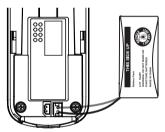
3. Slide the battery compartment cover towards the center of the handset until it clicks into place.
