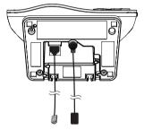
Position the lower portion grooves on the telephone base to the lower portion tabs (marked B) on the wall mount bracket. Make sure the upper portion grooves of the telephone base are above the upper portion tabs (marked A) on the wall mount bracket. Push the telephone base down until it clicks securely in place.
