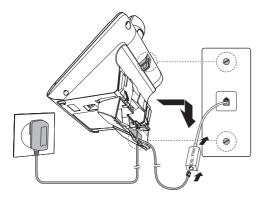
4. Slide the telephone base down until it clicks securely in place. Bundle the telephone line cord and power adapter cord neatly with twist ties if necessary.
