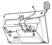
2. Press down on the tabs on the wall mount bracket on the telephone base to release it from tabletop orientation. Rotate the wall mount bracket down to wall mount position and then push it into the telephone base until it clicks into place.
