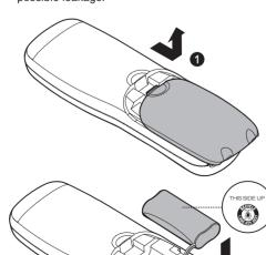
Install the battery as shown below.
