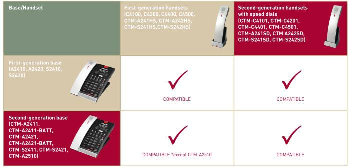
Note: Analog handsets only register to analog bases. SIP handsets only register to SIP bases.
