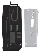
3. Install the telephone base as shown below. Then connect the coiled handset cord to the telephone base.
