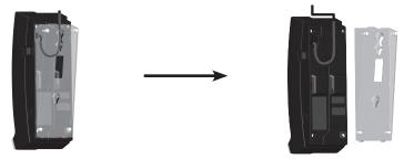
3. Turn the mounting bracket upside down. Remove the telephone line cord from the wire duct and then route it through the groove on the bottom part the mounting bracket. Insert the small tabs on the mounting bracket into the upper slots on the telephone base. Then press the large tab on the mounting bracket and firmly push it into the lower groove on the telephone base.
