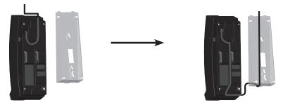
4. Mount the telephone base on the wall by aligning the eyelets with the mounting studs of the wall plate. Then slide the telephone base down on both mounting studs until it locks into place. Place the handset on the telephone base cradle.
