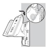
4. Connect the power adapter to the telephone base and an electrical outlet not controlled by a wall switch.
