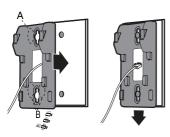
3. Align the grooves on the telephone base with the tabs on the wall mount bracket, and then slide it down until it clicks securely in place.
