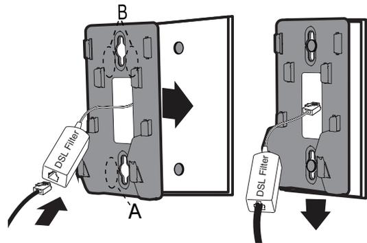
3. Align and place the telephone base on the wall mount bracket, and then connect the power adapter.
