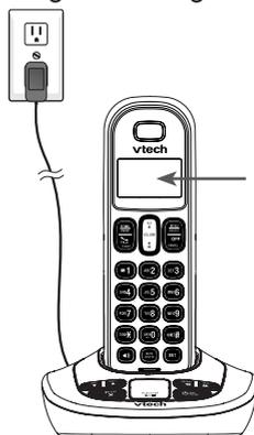
The LCD backlight turns on for 10 seconds to denote the battery starts to charge.
