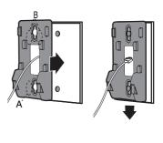
3. Align the grooves on the telephone base with the tabs on the wall mount bracket, and then slide it down until it clicks securely in place.
