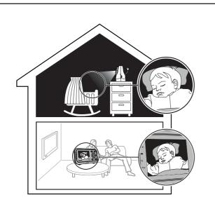
The baby unit has infrared LEDs that allow you to see your baby at night or in a dark room. When the baby unit detects low light levels, the infrared LEDs turn on automatically. The images from this baby unit is in black and white, and are appears on screen.
