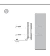
Align the wall mount bracket and screws with the holes in the wall as shown. Tighten the screw in the middle hole first, so that the wall mount bracket position is fixed. You can tighten the other screw in the top hole.
