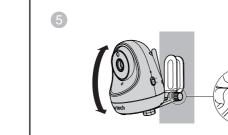
You can maximize your baby unit's viewing angles by tilting the wall mount bracket.
