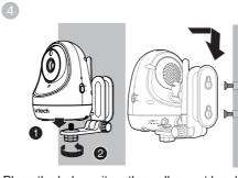
Place the baby unit on the wall mount bracket. Tighten the screw into the threaded socket at the bottom to secure the baby unit. Align the holes on the wall mount bracket with the screws on the wall, and slide the wall mount bracket down until it locks into place.
