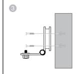
Align the wall mount bracket and screws with the holes in the wall as shown. Tighten the screw in the middle hole first, so that the wall mount bracket position is fixed. You can tighten the other screw in the top hole.
