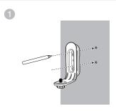
Check for reception strength and camera angle before drilling the holes.
