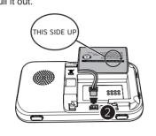
Make sure the label THIS SIDE UP is facing up while inserting the battery.
