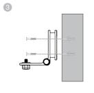
Align the wall mount bracket and screws with the holes in the wall as shown. Tighten the screw in the middle hole first, so that the wall mount bracket position is fixed. You can tighten the other screw in the top hole.
