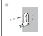
Check for reception strength and amera angle before drilling the holes.
