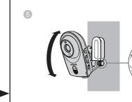
The default angle of the wall mount bracket is 90 degrees. You can maximize your baby unit's viewing angles by tilting the wall mount bracket.
