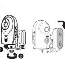
Place the baby unit on the wall mount bracket. Tighten the screw into the threaded socket at the bottom to secure the baby unit. Align the holes on the wall mount bracket with the screws on the wall, and slide the wall mount bracket down until it locks into place.
