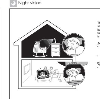
The baby unit has infrared LEDs that allow you to see your baby at night or in a dark room. When the baby unit detects low light levels, the infrared LEDs turn on automatically. The image from this baby unit is in black and white, and  $\supset$  appears on screen.
