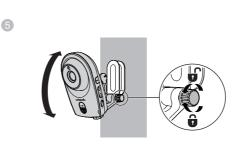
The default angle of the wall mount bracket is 90 degrees. You can maximize your baby unit's viewing angles by tilting the wall mount bracket.
