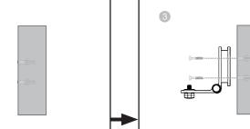
Align the wall mount bracket and screws with the holes in the wall as shown. Tighten the screw in the middle hole first, so that the wall mount bracket position is fixed. You can tighten the other screw in the top hole.
